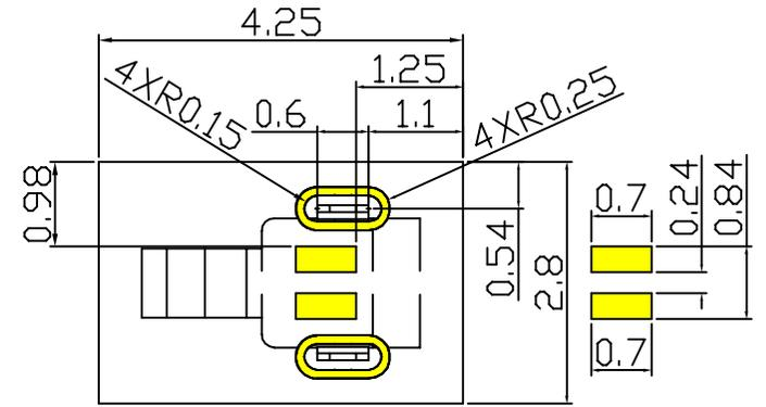
RECOMMENDED SOLDERING PCB LAYOUT
